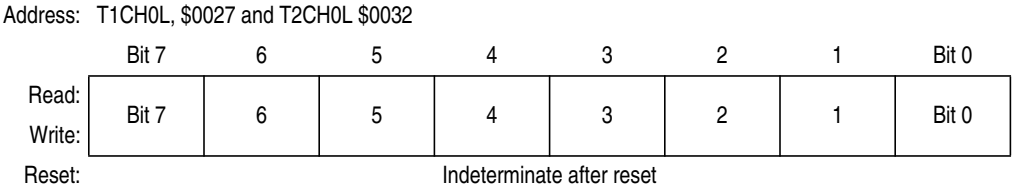
Figure 9-13. TIM Channel 0 Register Low (TCH0L)
