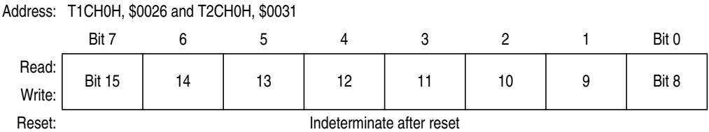
Figure 9-12. TIM Channel 0 Register High (TCH0H)
