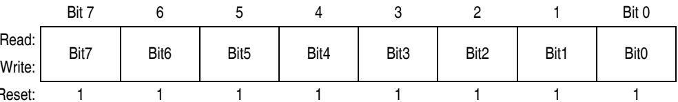
Figure 14-8. TIM Counter Modulo Low Register (TMODL)
