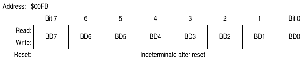
Figure 15-16. BDLC Data Register (BDR)
