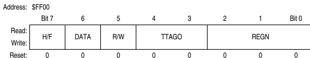
Figure 18-5. BDM Instruction Register (INSTRUCTION)
