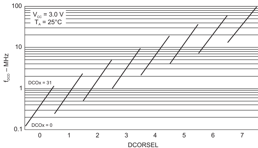
Figure 5-10. Typical DCO Frequency
