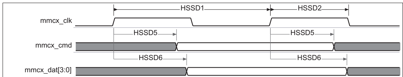
Figure 6-65. MMC/SD/SDIO – High-Speed SD Mode – Data/Command Receive
