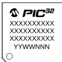
64-Lead TQFP (10x10x1 mm)
