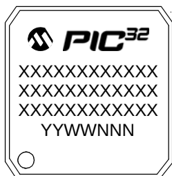
144-Lead TQFP (16x16x1 mm)
