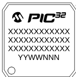
144-Lead TQFP (16x16x1 mm)
