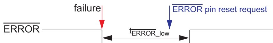
Figure 12-5. \overline{\text{ERROR}} Pin Timing - Example 2
