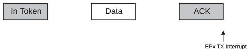
Figure 29-51. Non-Isochronous, Non-Control OUT Transaction Phases and Interrupts
