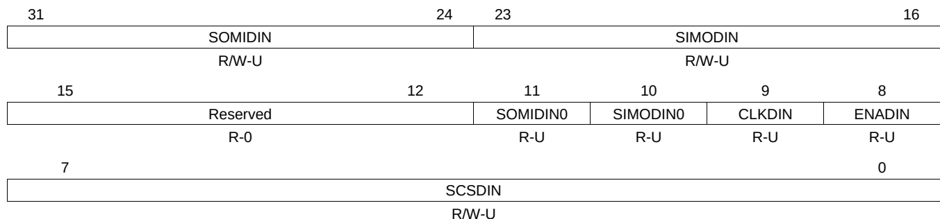
Figure 24-33. SPI Pin Control Register 2 (SPIPC2) [offset = 1Ch]
