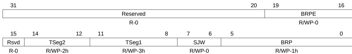
Figure 23-22. Bit Timing Register (DCAN BTR) [offset = 0Ch]
