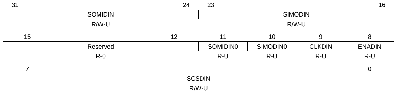
Figure 24-33. SPI Pin Control Register 2 (SPIPC2) [offset = 1Ch]
