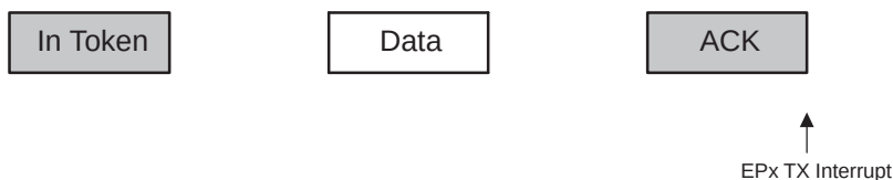
Figure 29-52. Non-Isochronous IN Transaction Phases and Interrupts
