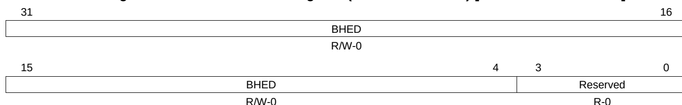
Figure 29-11. HC Head Bulk Register (HCBULKHEADED) [address = FCF78B28h]
