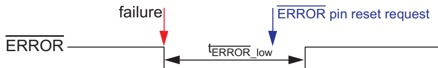
Figure 12-5. \overline{\text{ERROR}} Pin Timing - Example 2
