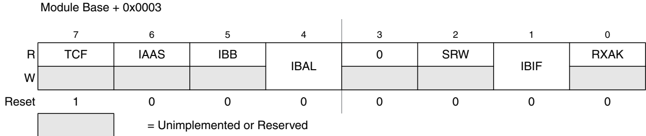
Figure 15-7. IIC Bus Status Register (IBSR)
