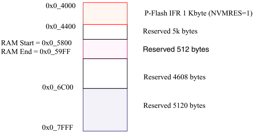
Figure 26-3. Memory Controller Resource Memory Map (NVMRES=1)
