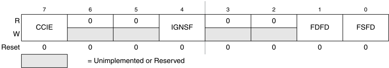
Figure 24-9. Flash Configuration Register (FCNFG)
