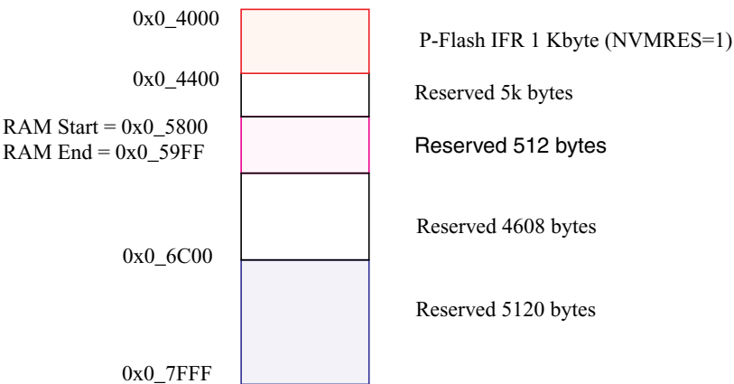
Figure 29-3. Memory Controller Resource Memory Map (NVMRES=1)
