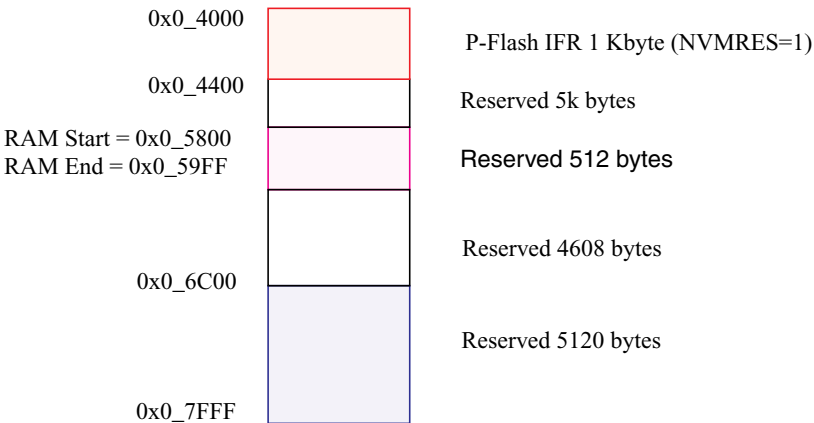
Figure 29-3. Memory Controller Resource Memory Map (NVMRES=1)
