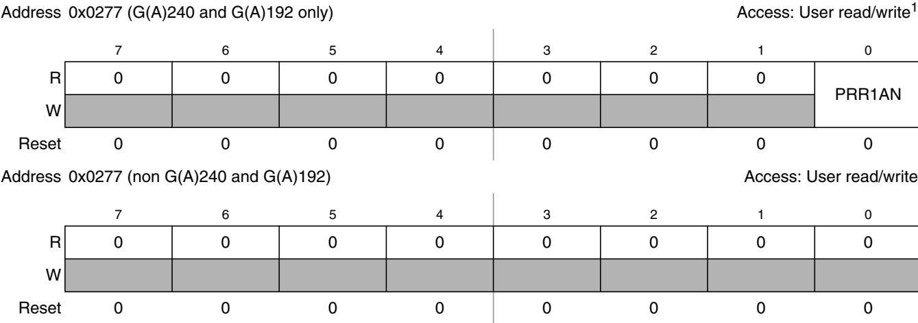
Figure 2-55. Pin Routing Register (PRR1)
