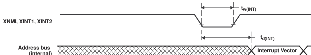
Figure 7-15. External Interrupt Timing
