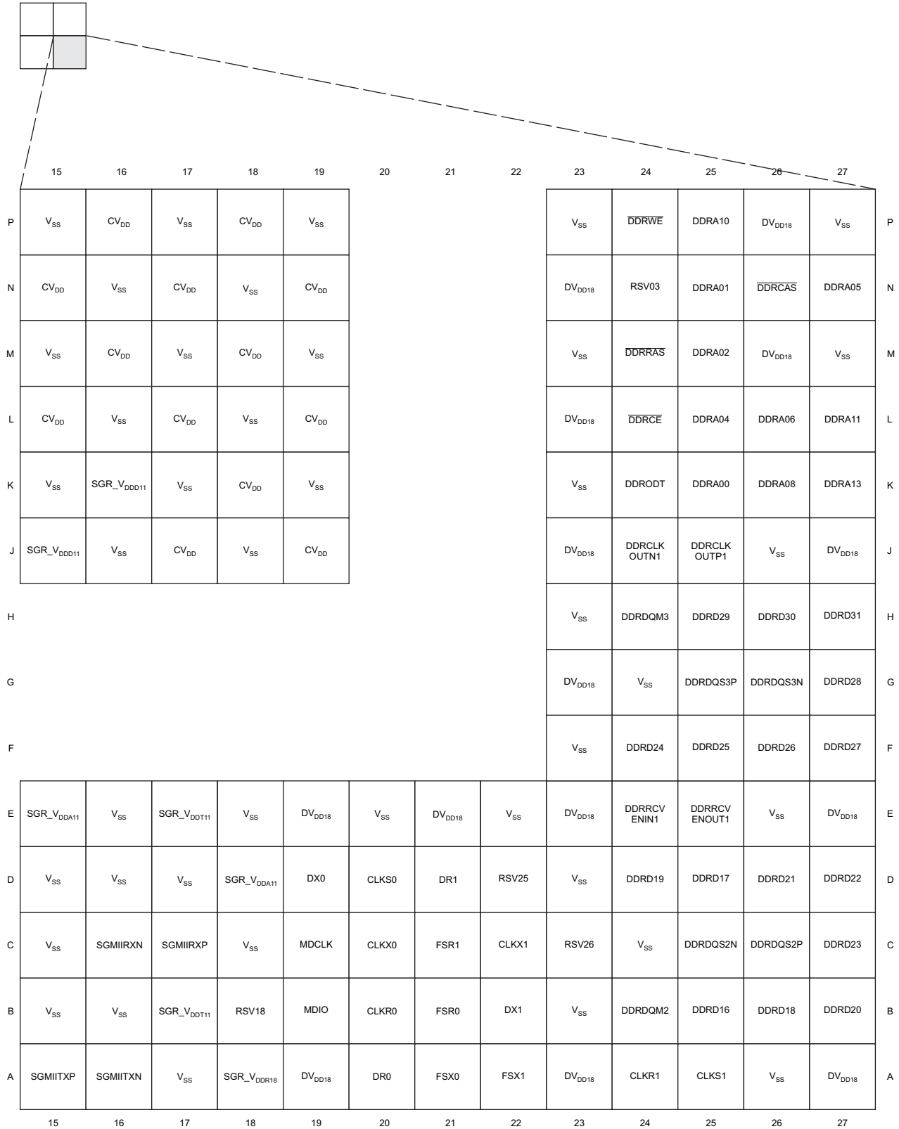
Figure 2-4. C6474 Pin Map (Bottom View) [Quadrant C]
