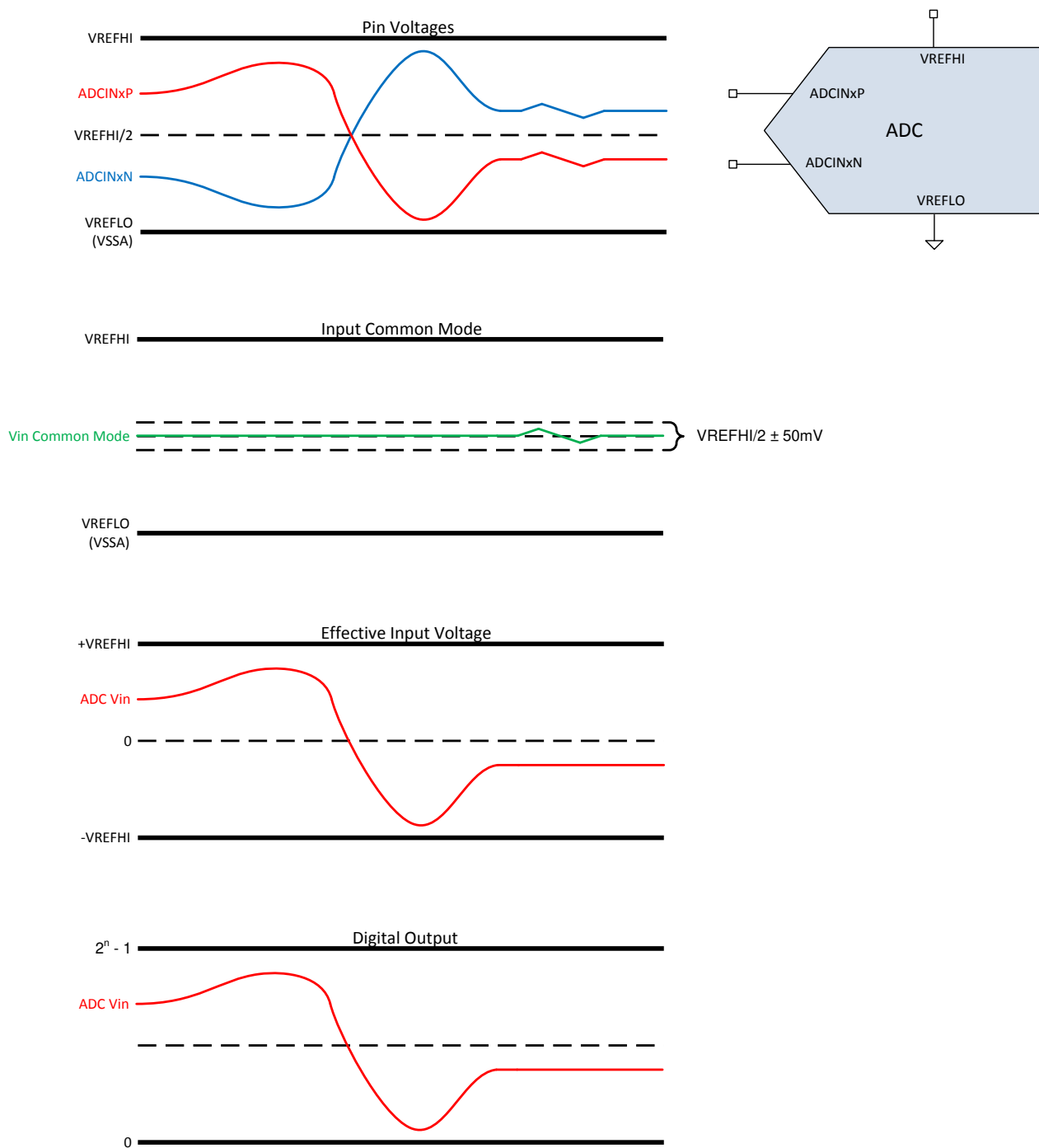
Figure 6-35. Differential Signaling Mode
