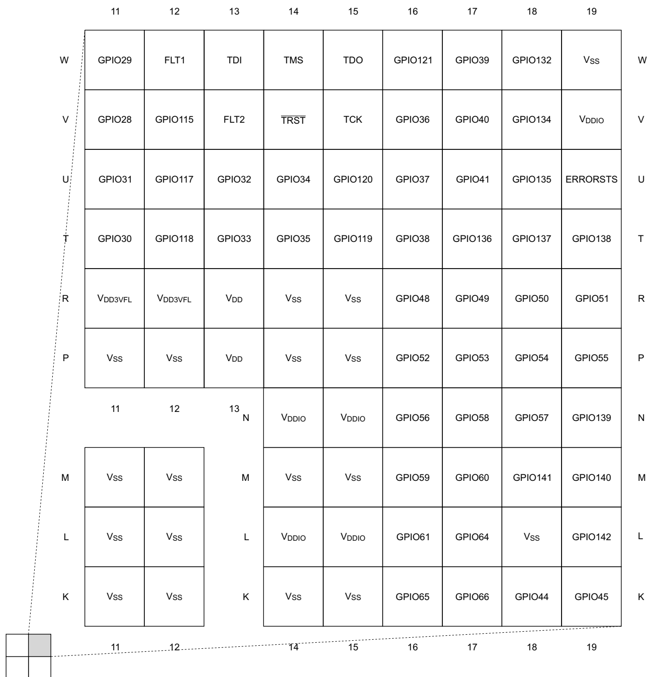
Figure 5-2. 337-Ball ZWT New Fine Pitch Ball Grid Array (Bottom View) – [Quadrant B]
