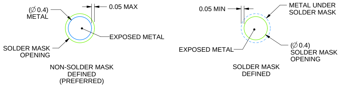
SOLDER MASK DETAILS NOT TO SCALE
