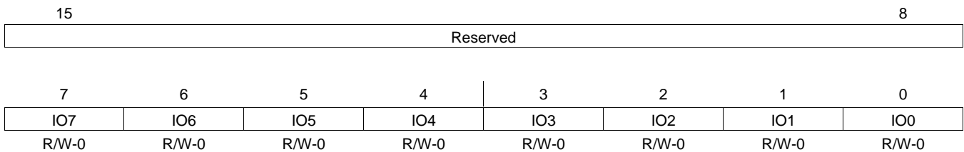
Figure 3-24. General-Purpose I/O Status Register (GPIOSR) [MMR Address 003Dh]
