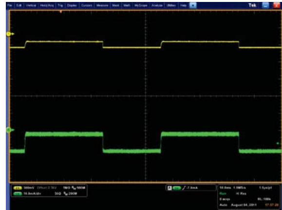
Figure 32. ZEROiddq Load Transient Response (0 to 10mA) Code 4, 1.4V drop. Ch1: VBAT, Ch3: VMICRO (LDO MINI output) (100mV/div). Ch4 Load current (10mA/div).
