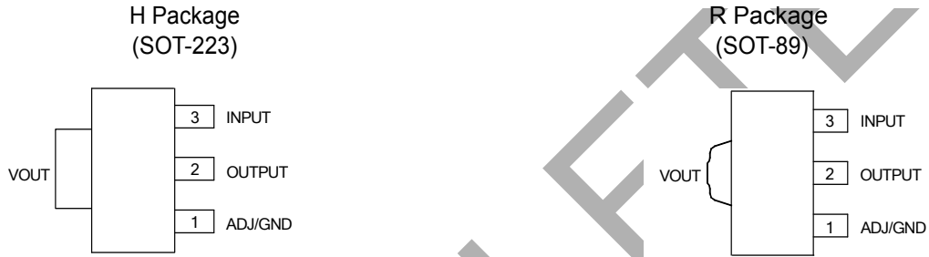
Figure 2. Pin Configuration of AZ1117B (Top View)
