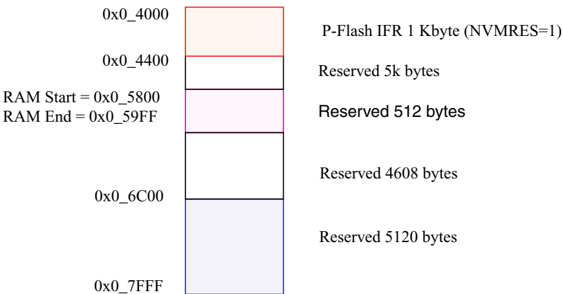
Figure 29-3. Memory Controller Resource Memory Map (NVMRES=1)
