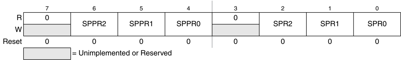
Figure 21-5. SPI Baud Rate Register (SPIBR)
