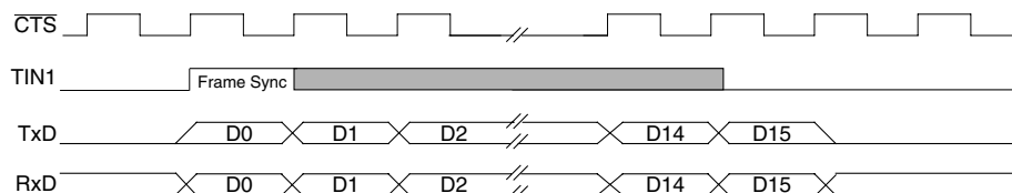
Figure 14-31. 16-Bit CODEC Interface Timing (lsb First)
