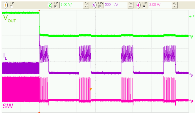
Figure 33. Metallic Short Applied at V_{OUT} , 50\ \mu\text{s}/\text{div} .
