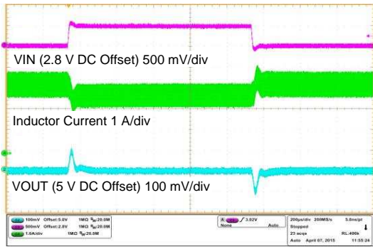
VIN = 2.8 V to 3.3 V, VOUT = 5 V, IOU = 2 A
