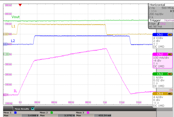
Figure 8-11. Switching Waveforms, Boost Operation
