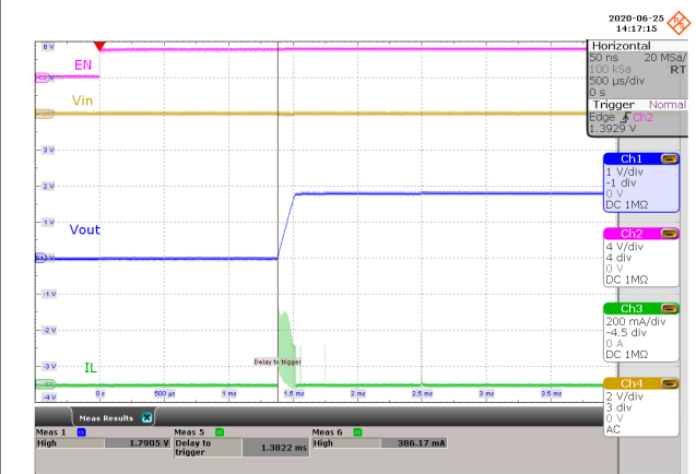
Figure 8-27. Load Transient, 300 mA Step
