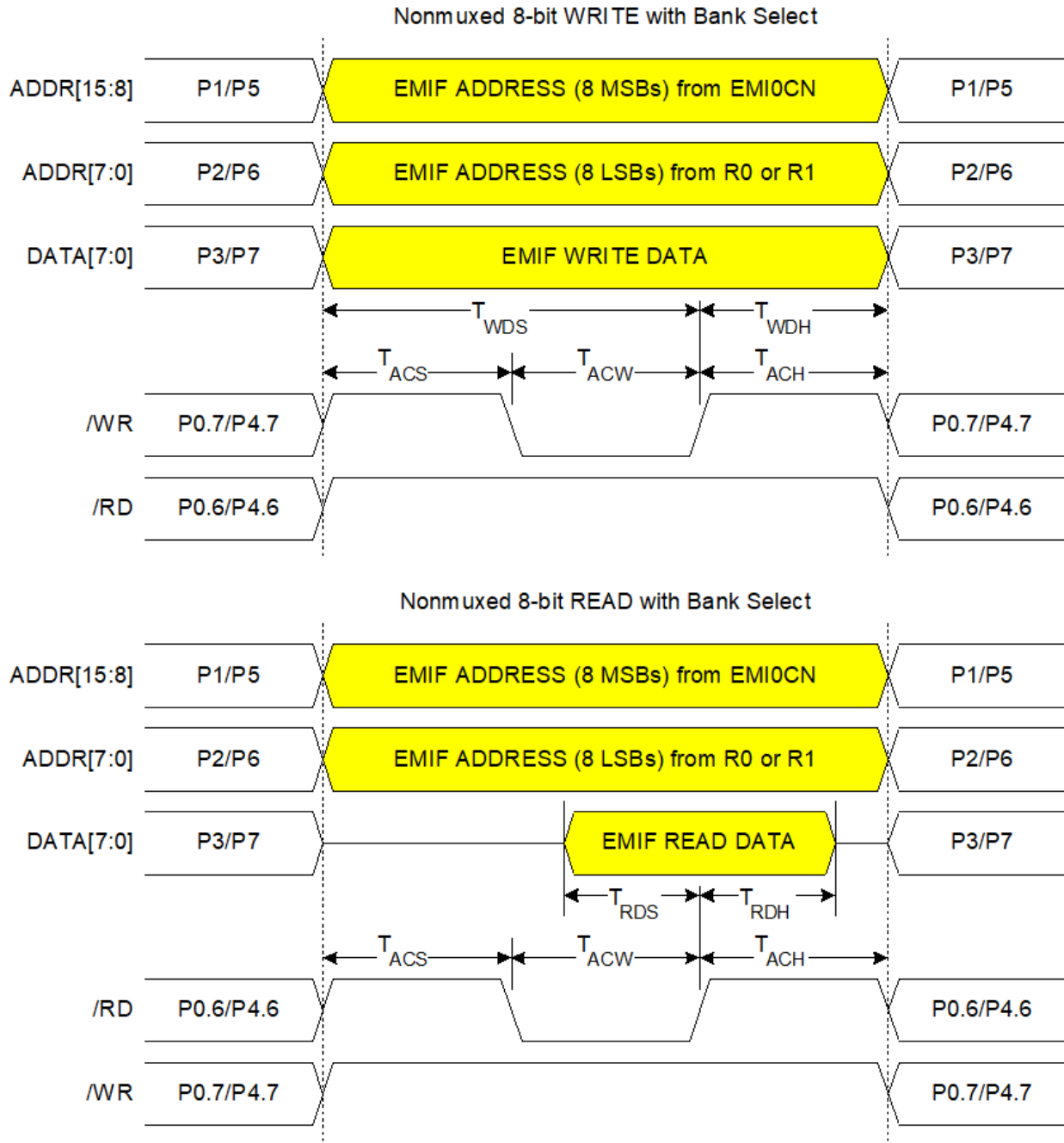
Figure 17.6. Non-multiplexed 8-bit MOVX with Bank Select Timing
