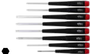
8 Pc. Precision Ball End Hex Inch Driver Set Item No. Description Case Pack 26490 Prec. Ball End Hex Inch Set 3 Inch: .050, 1/16, 5/64, 3/32, 7/64, 1/8, 9/64, 5/32"
