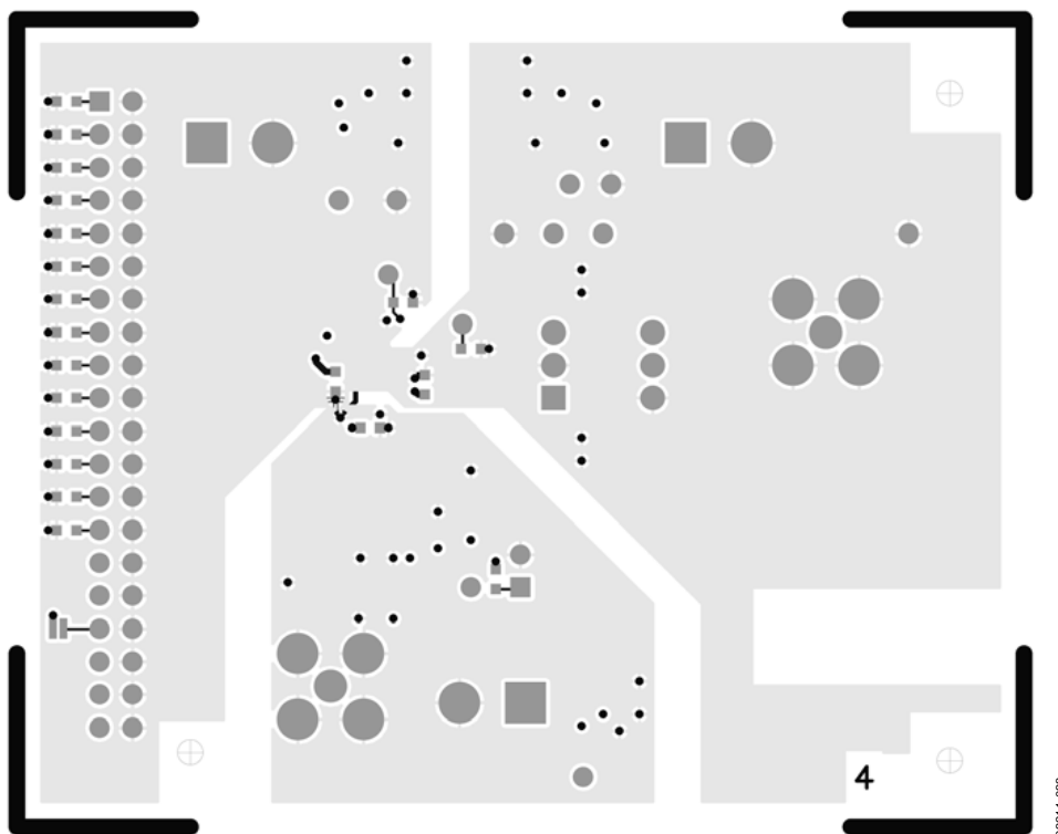
Figure 36. Evaluation Board Layout—Secondary Side
