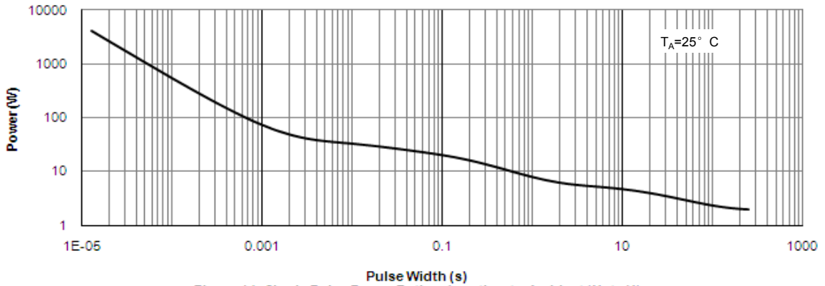
Figure 14: Single Pulse Power Rating Junction-to-Ambient (Note H)
