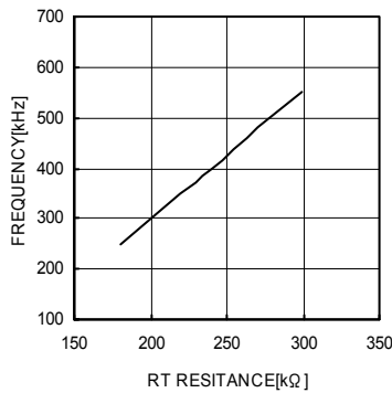
Figure 22. RT resistor vs. oscillation frequency
