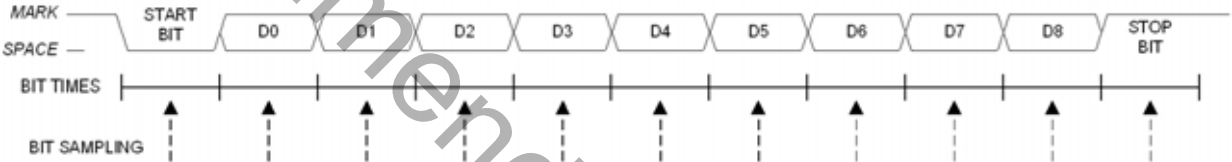
Figure 22.5. 9-Bit UART Timing Diagram
