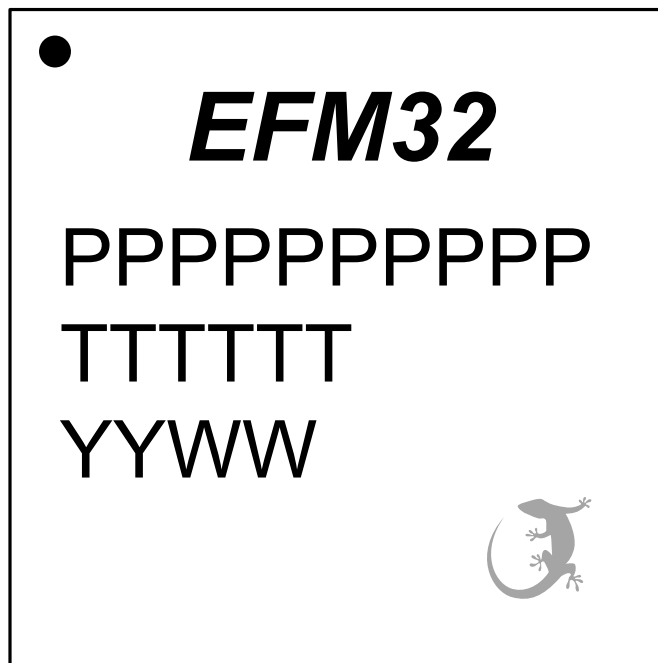
Figure 10.3. TQFP48 Package Marking
