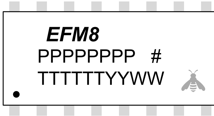
Figure 9.3. SOIC16 Package Marking
