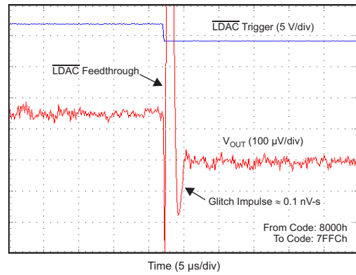
Figure 80. Glitch Impulse Falling Edge, 1-LSB Step
