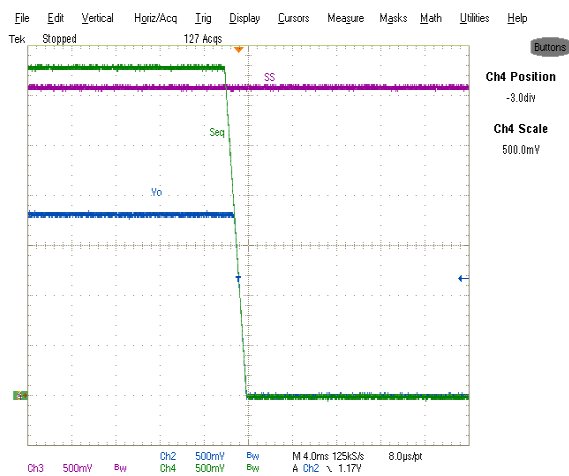
Fig. 25: Simultaneous Tracking a 3.3V input at power-up and shut-down Ch2: Vout Ch3:SS Ch4: Seq
