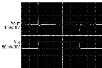
Input Voltage Line Transient Response
