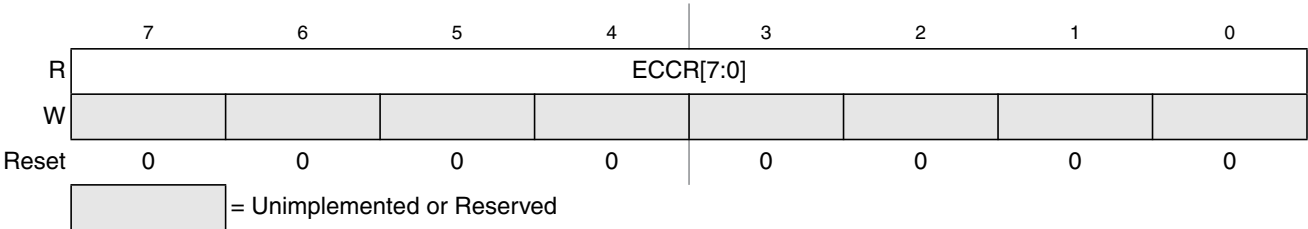
Figure 24-21. Flash ECC Error Results Low Register (FECCRLO)
