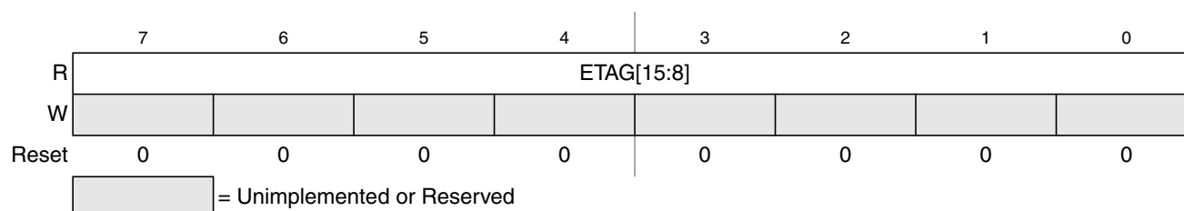
Figure 28-18. EEE Tag Counter High Register (ETAGHI)
