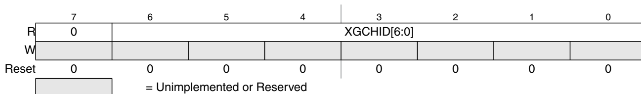
Figure 10-4. XGATE Channel ID Register (XGCHID)
