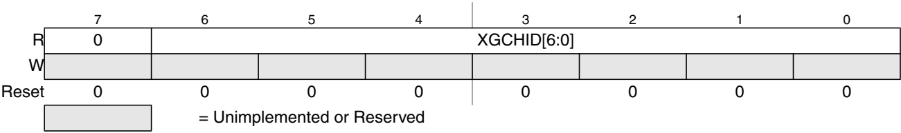
Figure 10-4. XGATE Channel ID Register (XGCHID)
