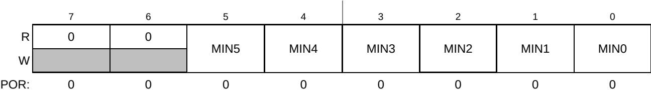
Figure 16-11. Minute Register (MINR)
