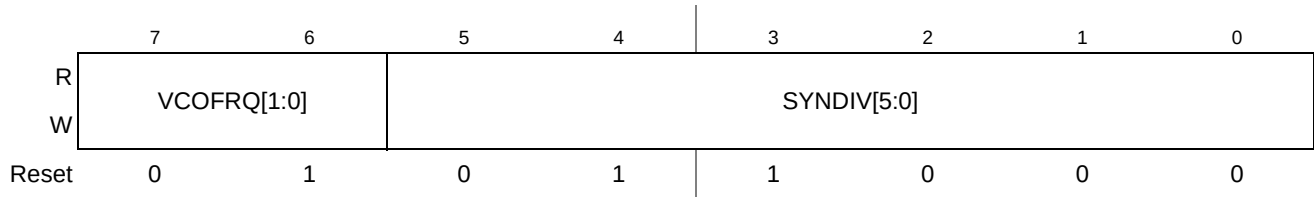
Figure 7-5. S12CPMU_UHV_V5 Synthesizer Register (CPMUSYNR)
