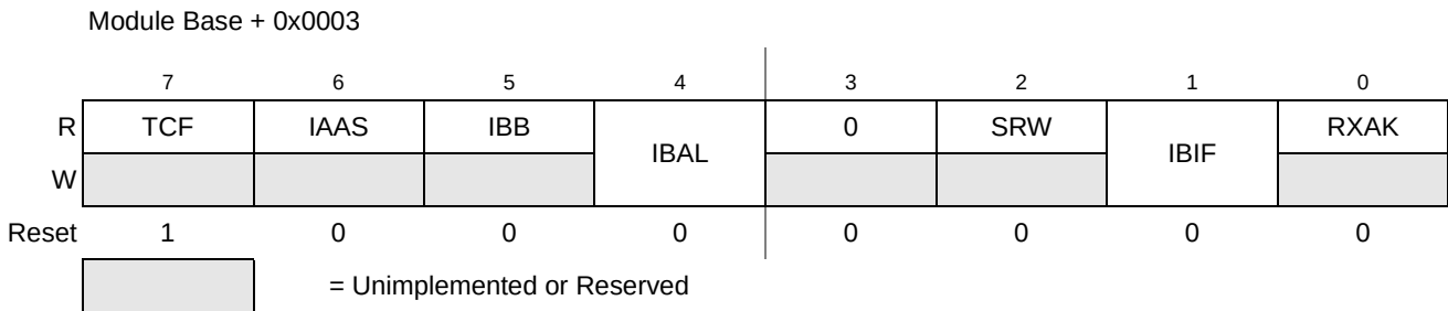
Figure 14-7. IIC Bus Status Register (IBSR)
