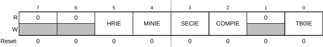
Figure 16-5. RTC Control Register 4 (RTCCTL4)
