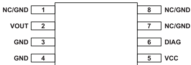
Package LE, 8-Pin eTSSOP Pinouts
