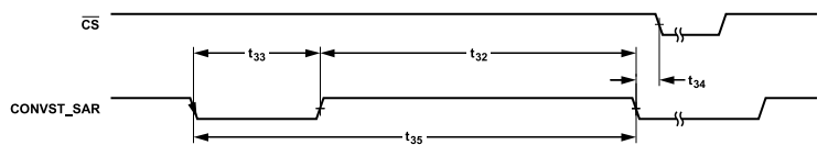
Figure 5. SAR ADC Timing Diagram
