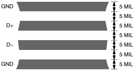
Figure 21. Typical Arrangement of Signal Tracks
