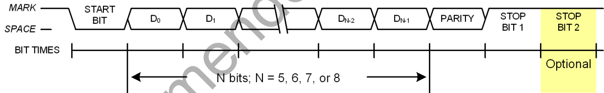
Figure 26.3. UART1 Timing With Parity
