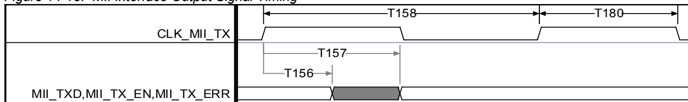
Figure 14-15. MII Interface Output Signal Timing
